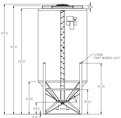
DRAWN / DATE MATERIAL ADH 10/14/19 TANK: HDPE OR EQUIVALENT APPRD. / DATE STAND: MILD STEEL REH 11/14/19 REV DESCRIPTION BY / DATE CCN ALL DIMENSIONS ARE IN DECIMAL INCHES SHOT WEIGHT: THIRD ANGLE PROJECTION NOTES: TOLERANCES UNLESS OTHERWISE SPECIFIED DESCRIPTION SHIPPING WEIGHT: SEE NOTES . TANK WEIGHT 170.50 LBS POLYETHYLENE METAL DECIMAL ± .125" 2. STAND WEIGHT 174 LBS. SCALE ±1% @ 68°F FRACTION ± 1/4"
